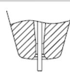
1. The bonding process begins with a threaded capillary.
