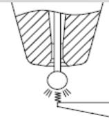
2. Electrical Flame Off (EFO) forms the free air ball.
